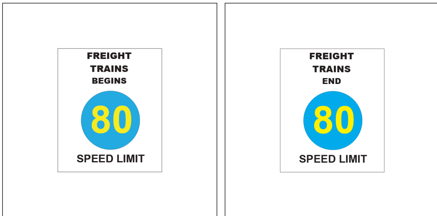
FIGURE 50: Freight train speed signs.
