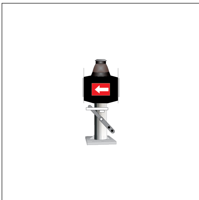
FIGURE 8: Example of a mechanical point indicator shows points are set for the route indicated by the direction of the arrow.
