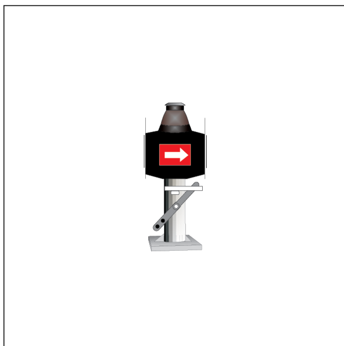
FIGURE 8: Example of a mechanical point indicator shows points are set for the route indicated by the direction of the arrow.
