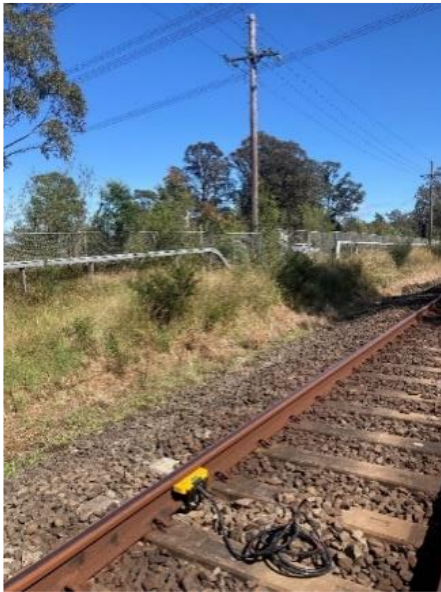
Image 1: Transmitter and sensor installation location
