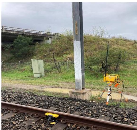
Image 1: Transmitter and sensor installation location
