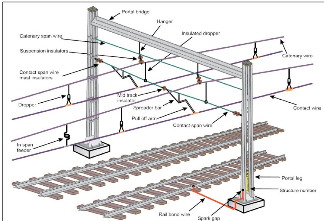
**Figure 1: Simple catenary, fixed anchored, span wire construction on portal structures**
