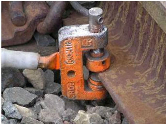
**Figure 3: Partially engaged clamp (no good)**
