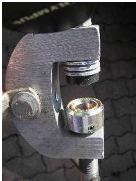
**Figure 1: Condition of a good clamp**
