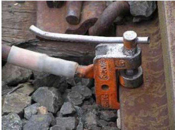
**Figure 2: Fully engaged clamp**
