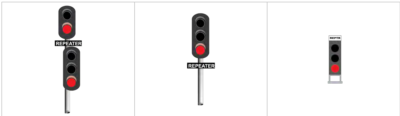
FIGURE 13: Colour light repeater signals.
