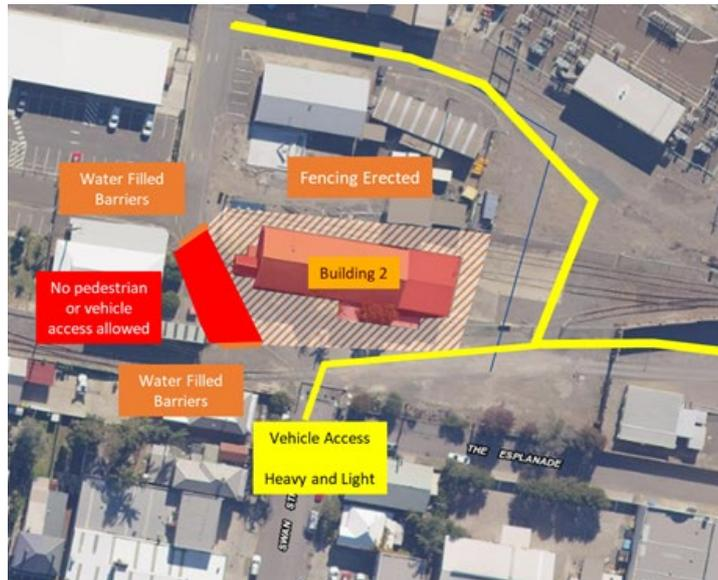
**Figure 1:** Illustrates the changes to traffic flow and placement of barriers to prevent access.
