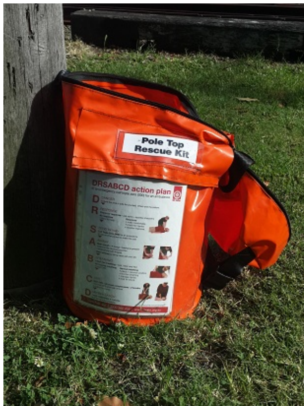
Photo 2: Pole Top Rescue Kit at Bottom of Pole
