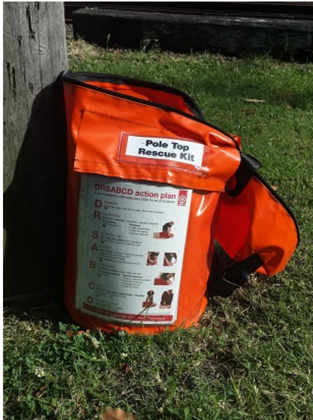
Figure 2 – Pole Top Rescue Kit at Bottom of Pole
