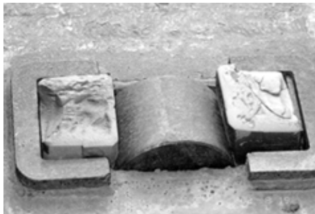
Figure 3: Constant contact side bearers with melted plastic blocks
