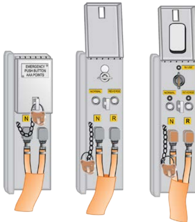
FIGURE 2: Control box operated by an EOL key
