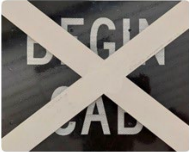
Example Begin In-Cab Signalling Sign fitted with White X
