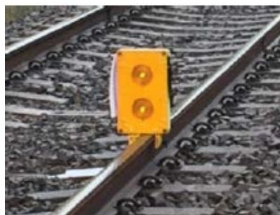
FIGURE 2: Dual light Worksite Delineation Marker clamped to the rail.
