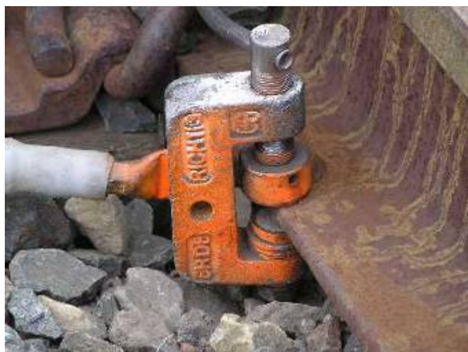
Partially Engaged Clamp (no good)
