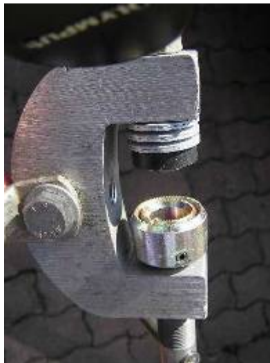
Condition of a Good Clamp
