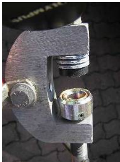
Figure 1 – Condition of a good clamp
