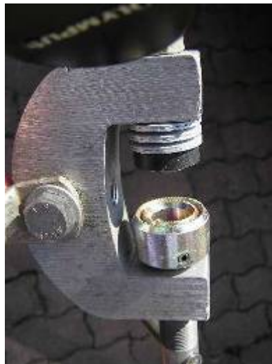
Condition of a Good Clamp
