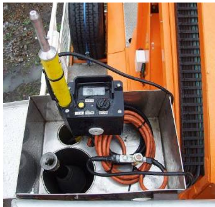
Negative Lug Attached to an Approved Rail Connection Bolt on an EWP
