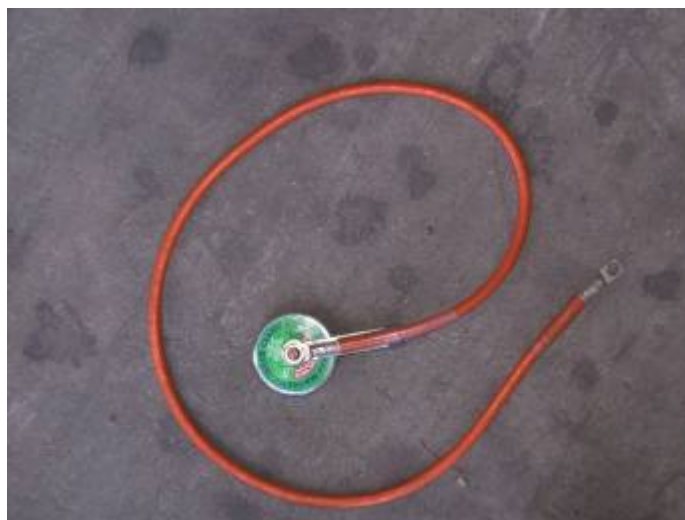
Welder's Magnetic Clamp Assembly (This assembly is for use with the LR Tester, NOT the Hivotech 1500V DC OHW Tester.)
