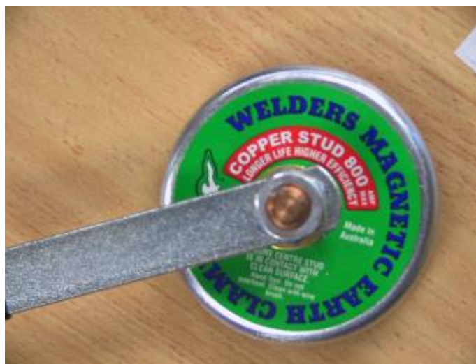
Welder's Magnetic Clamp (This assembly is for use with both the LR Tester & Hivotech 1500V DC OHW Tester)
