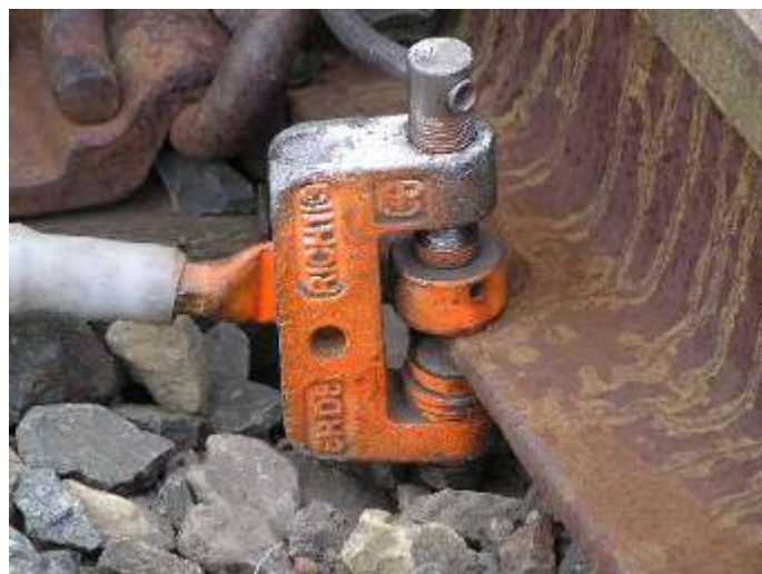
Partially Engaged Clamp (no good)
