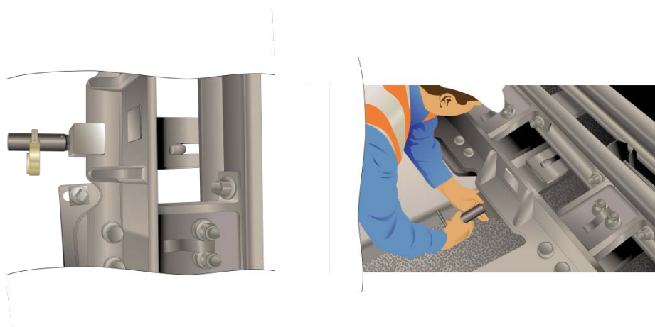
FIGURE 4: Example of a point clip fitted to the swingnose of VAE Points. This type of point uses a special point clip fitted to a plate under the movable swingnose of the points.
