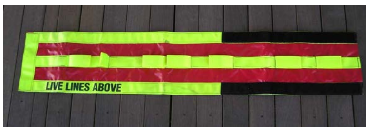
Figure 1 A suitable pole marker
