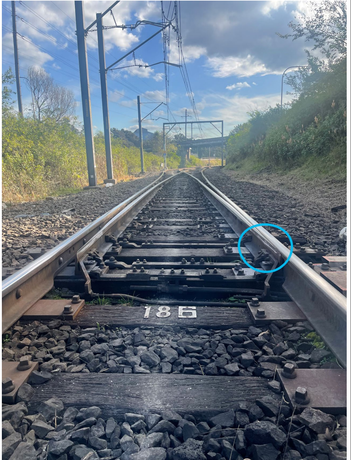
Image 2: Port Kembla Side TOA Limits 186 Points (Point Clip position circled)
