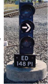
POINT INDICATOR WITH ILLUMINATED ARROW
