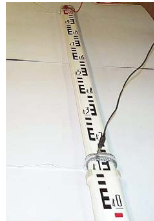
Figure 5 Views of attachment of braid and position of test leads for IR tests on one section of the white telescopic stave.
