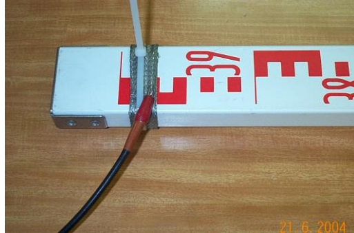
Figure 6 Views of attachment of braid to top section of a white three-section telescopic stave
