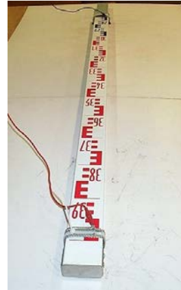
Figure 6 Views of attachment of braid to top section of a white three-section telescopic stave
