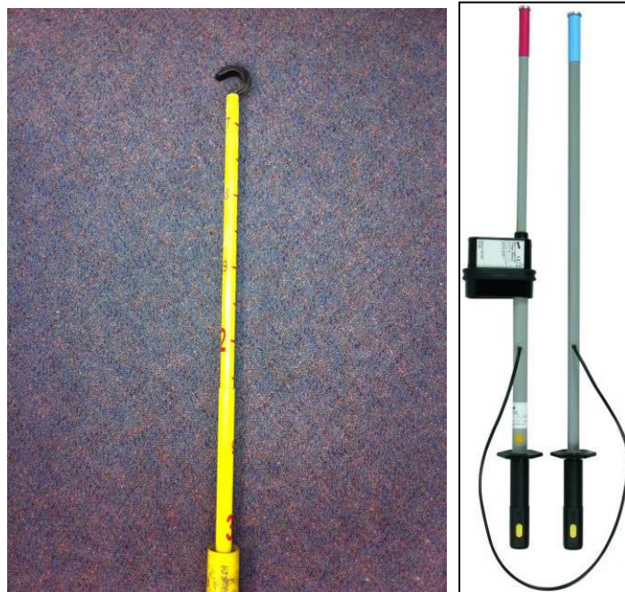
Figure 2 Dedicated 1500V DC Telescopic Height Measuring Stick & Dehn PHE/GII 1500V DC Substation Voltage Detector – Used for working "On"
