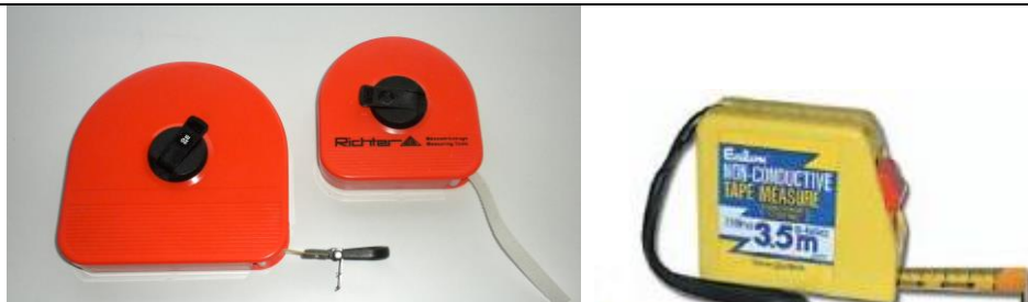
Figure 3 Only non-conductive tape measures to be used within the rail corridor
