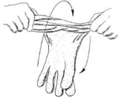
Step 2. Twirl Glove Towards Your Body to Trap Air Inside. Squeeze Glove To Look For Damage.
