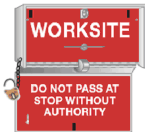
FIGURE 1: Opened Signal Key Switch Box
