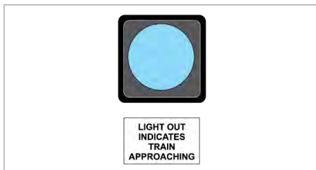
FIGURE 12: Example of a crossing light.
