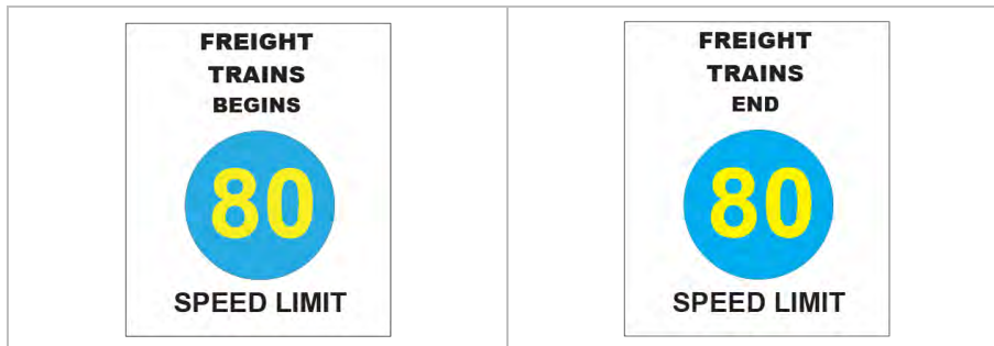
FIGURE 50: Freight train speed signs.
