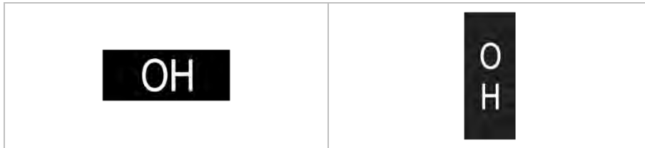
FIGURE 39: Examples of distant signal designation plates.
