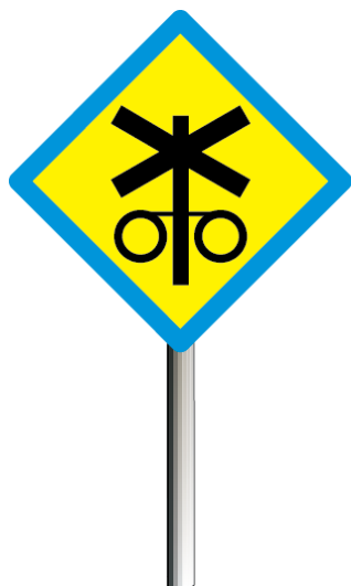
FIGURE 4: Trackside sign before Type F level crossing within predictor circuitry
