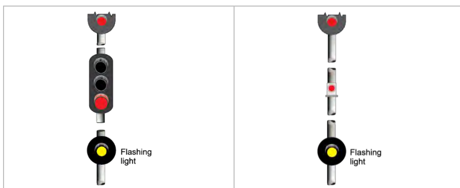
FIGURE 10: Examples of shunt ahead signals displaying PROCEED.
