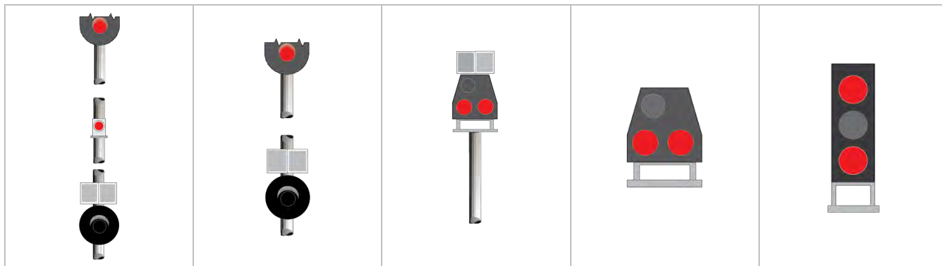
FIGURE 4: Examples of semaphore shunting signals displaying PROCEED.
