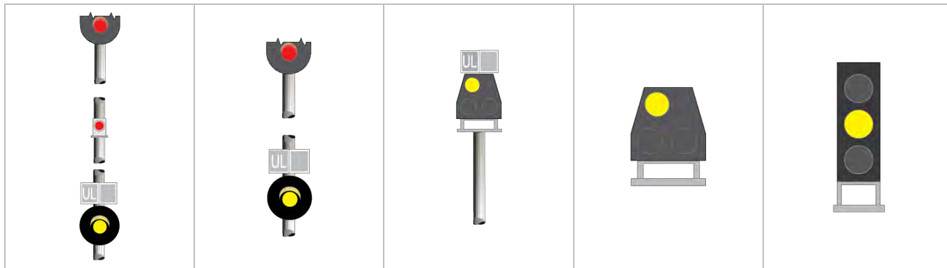
FIGURE 3: Examples of colour light shunting signals displaying STOP.
