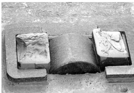
Figure 3: Constant contact side bearers with melted plastic blocks
