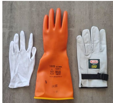
Insulated glove with cotton inner and leather/rigger glove outer
