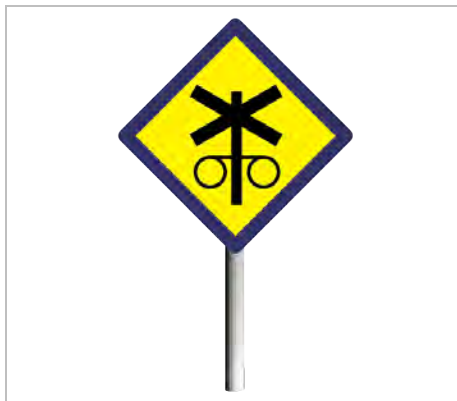
FIGURE 4: Trackside sign before Type F level crossing within predictor circuitry
