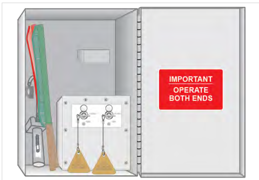
FIGURE 4: EOL cabinet with keys for two hand throw electric points machines.
