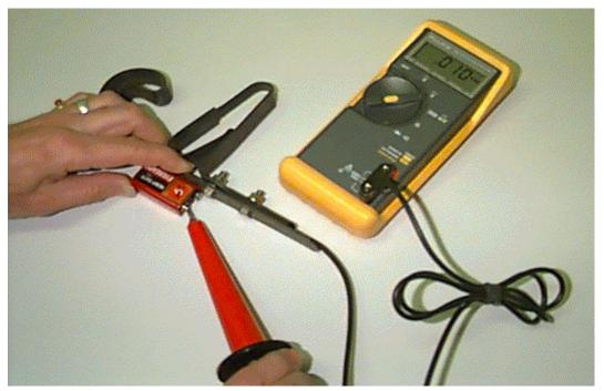
Hold the HV probe ③ on to the +ve terminal of the 9V battery ③ and the eye of the rail vehicle lead ⑥ on to the -ve terminal of the battery. The multimeter ① shall read between .011 and .007 VDC. The HV probe reduces the voltage 1000 times i.e. 9 V = .009 VDC on the multimeter.
