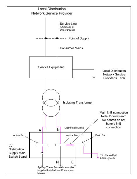
Figure 2: Station Supply from Local Distribution Network Service Provider (Main elements ONLY shown)
