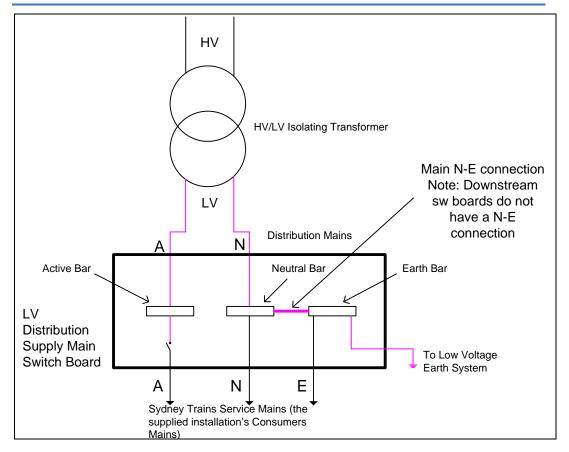
Figure 1: Supply from TAHE High Voltage Network (Main elements ONLY shown)
