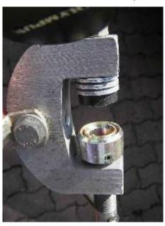
Figure 1: Condition of a good clamp
