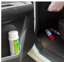
Aerosol cans not stored correctly. All Hazardous substances should be stored as per their Safety Data Sheet and not in the cabin of the vehicle.
