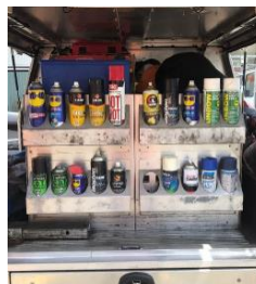
Aerosol cans stored correctly in the rear of vehicle and in correct holders.
