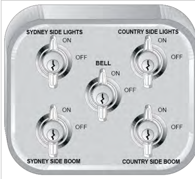
FIGURE 7: Emergency switch box with individual switches for lights, bell, and booms.
