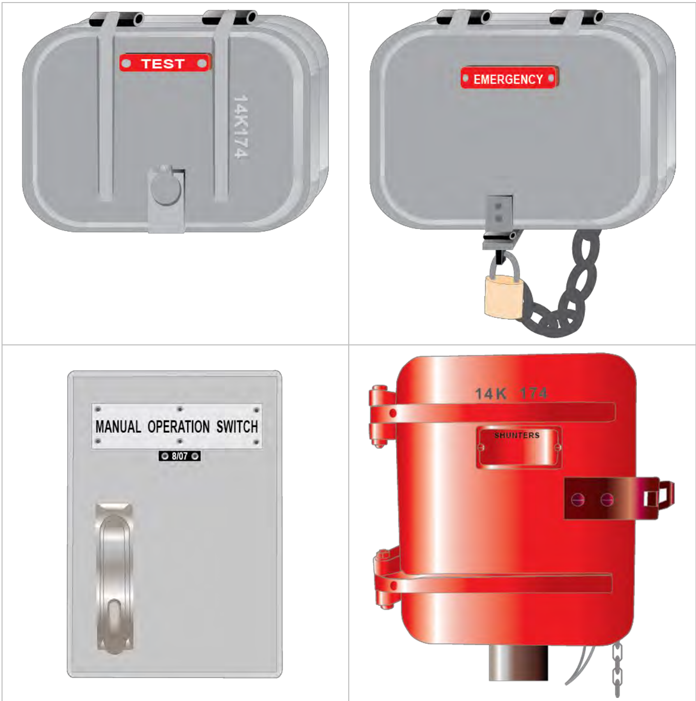
FIGURE 2: Level crossing switch boxes
