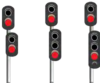
FIGURE 6: Staggered colour light forms
