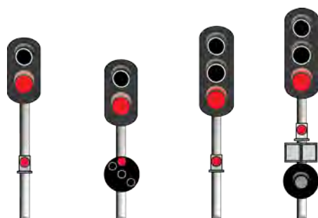
FIGURE 9: Single head signal forms
