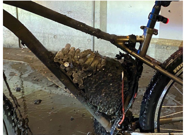
Figure 1: e-bike damage following battery thermal runaway fire
