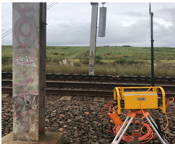
Image 1: Transmitter and sensor installation location
