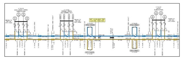
Figure 5: A typical sectioning arrangement between two substations
