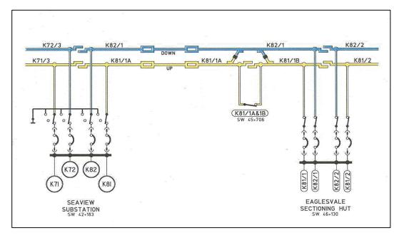
Figure 4: Sectioning diagram for a two track arrangement between a substation and a sectioning hut
