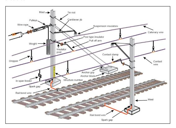
Figure 2: Simple catenary, regulated tension, cantilever construction on masts
