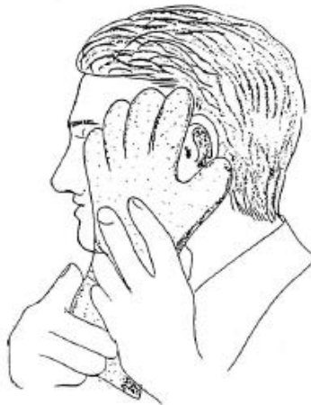
Step 3. Hold Glove To Face and Feel. Listen For Escaping Air or Immerse In Water and Watch For Bubbles.
