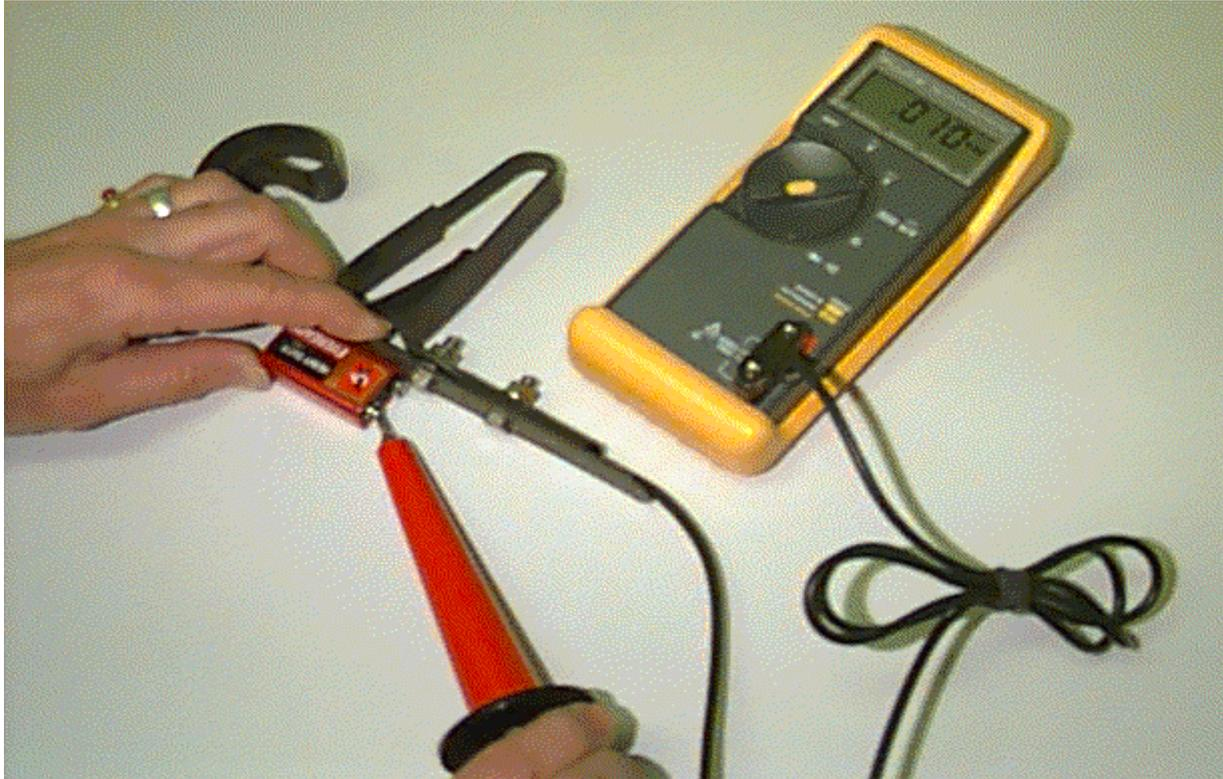
Hold the HV probe ③ on to the +ve terminal of the 9V battery ⑧ and the eye of the rail vehicle lead ⑥ on to the -ve terminal of the battery. The multimeter ① shall read between .011 and .007 VDC. The HV probe reduces the voltage 1000 times
