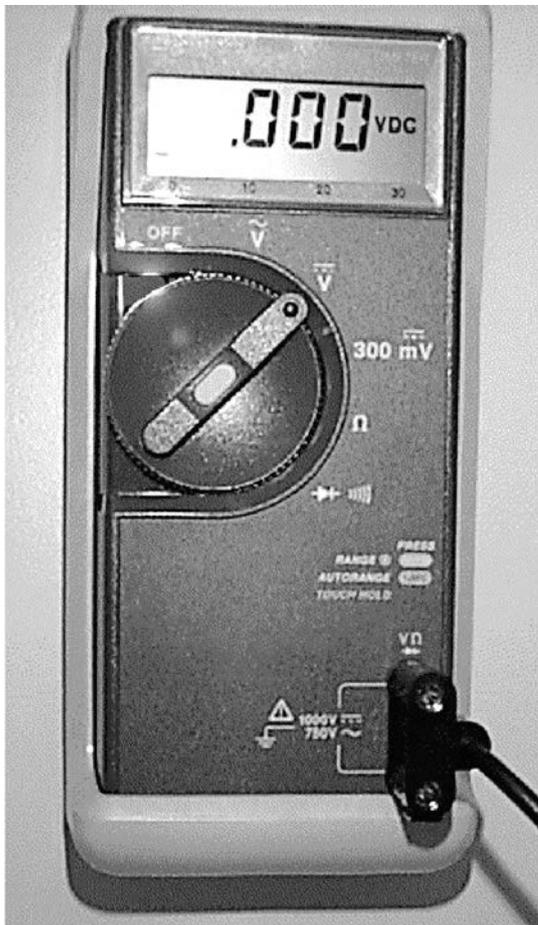
The plug pin next to the "GND" lug shall be in the "COM" socket (the bottom hole). The lead plug housing will then be on the outside of the multimeter. The multimeter should show .000 VDC.
