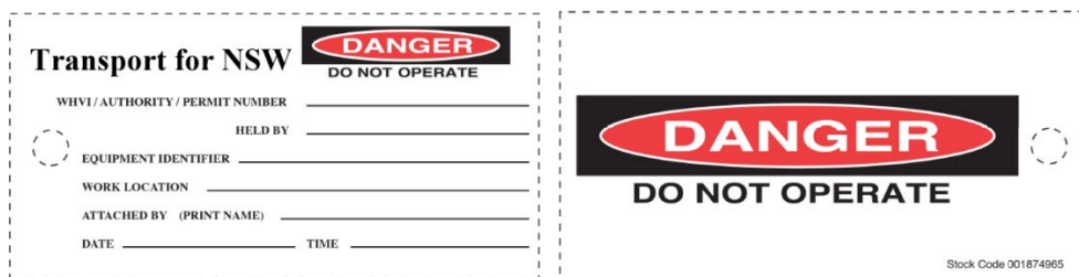
Figure 2 Example front and back of a 'blank' DANGER Tag (Stock Code: 001874965)
