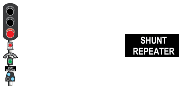
FIGURE 7: At left, the shunt repeater signal shows that the next shunting signal displays PROCEED. At right, a shunt repeater sign
