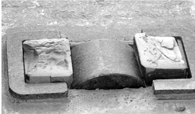
Figure 3: Constant contact side bearers with melted plastic blocks
