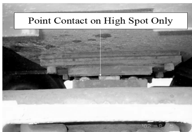
Figure 1: High gib/side frame wear and friction wedge lateral wear
