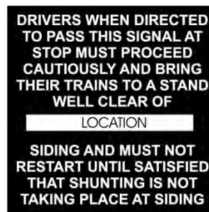
FIGURE 30: Example of intermediate siding sign
