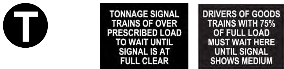
FIGURE 27: Tonnage indicator and examples of instruction signs
