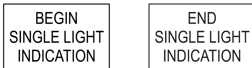
FIGURE 38: Begin and end single light indication signs
