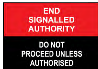
FIGURE 21: Example of END SIGNALLED AUTHORITY sign .....
