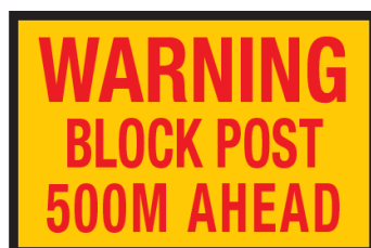
FIGURE 14: Example of a BLOCK POST WARNING sign
