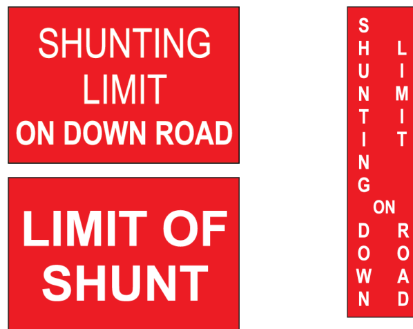
FIGURE 33: Examples of SHUNTING LIMIT signs
